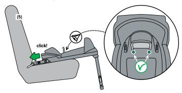
**5-** Push the ISOfix release handle down in the base. Push the ISOfix base as far as possible towards the backrest of the vehicle seat (6).
