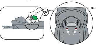
**3-** Push the ISOfix release handle down (12). Push the ISOfix anchorages totally inside the base (13).
