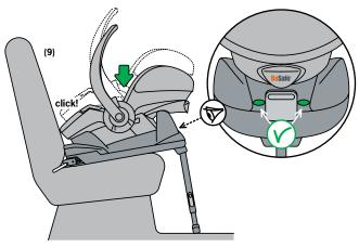
Leave the carrying handle of the seat in the vertical position carrying position while driving.
