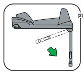
**3-** Pull the ISOfix release handle to a vertical position (3). Slide the ISOfix connectors out of the base till the end stop (4).
