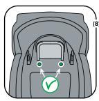
**8-** Position the iZi Go on the base. Check if the seat is fixed to the base and if the seat release indicators of the release handle indicate green (9). If the indicators do not indicate green, check if the seat is fixed in the right way.
